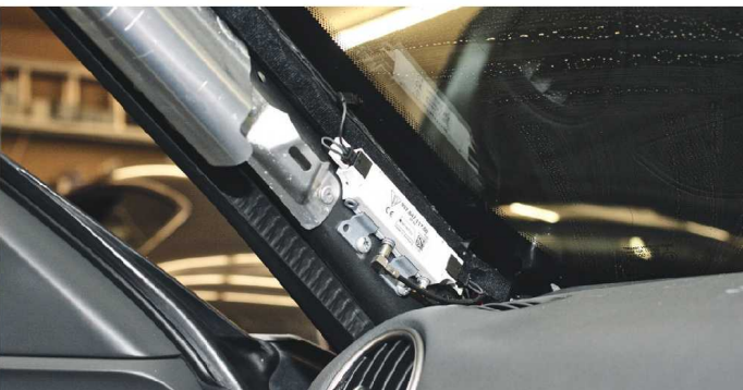
Above: New mic sits under the dash cowl for noise protection. Left: FM and DAB aerial fitment
