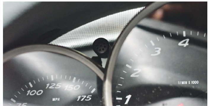
Above: New mic sits under the dash cowl for noise protection. Left: FM and DAB aerial fitment
